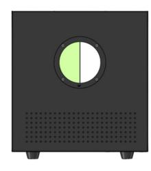
**LEDMax** is a precision trichromator that measures the three individual LMS cone spectral sensitivities through empirical color matching. Utilizing 2x18 multispectral LEDs (spanning 400 to 700nm) each illuminating one of two patented dual hemi-fields, the biometric visual data allow the mean theoretical CIE color standards to be replaced with precise individual functions, helping to eliminate observer metamerism across industries.
