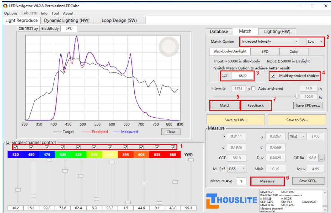
Fig. 6.6 manually intensity adjustment based match procedure
