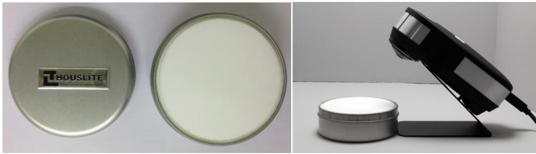
Fig. 4.2 An example of THOUSLITE standard white tile
