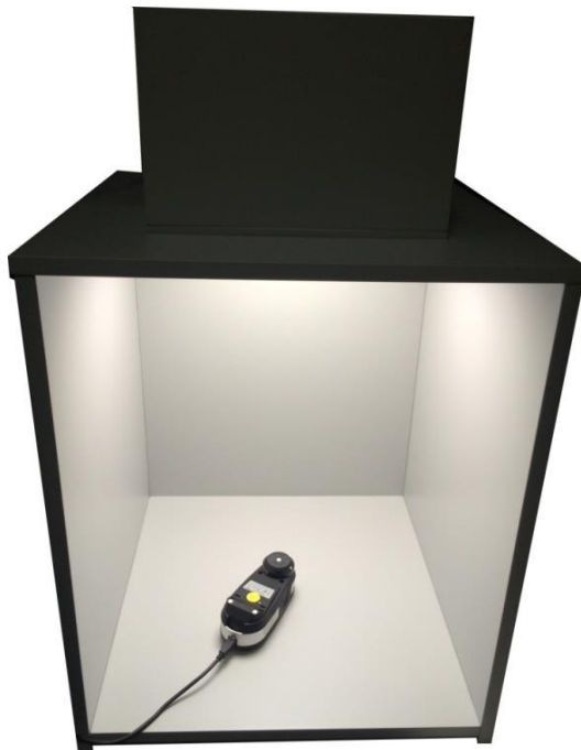
Fig. 4.15 i1 Pro2 with illumination head measurement position
