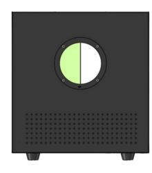
**LEDMax** is a precision trichromator that measures the three individual LMS cone spectral sensitivities through empirical color matching. Utilizing 2x18 multispectral LEDs (spanning 400 to 700nm) each illuminating one of two patented dual hemi-fields, the biometric visual data allow the mean theoretical CIE color standards to be replaced with precise individual functions, helping to eliminate observer metamerism across industries.
